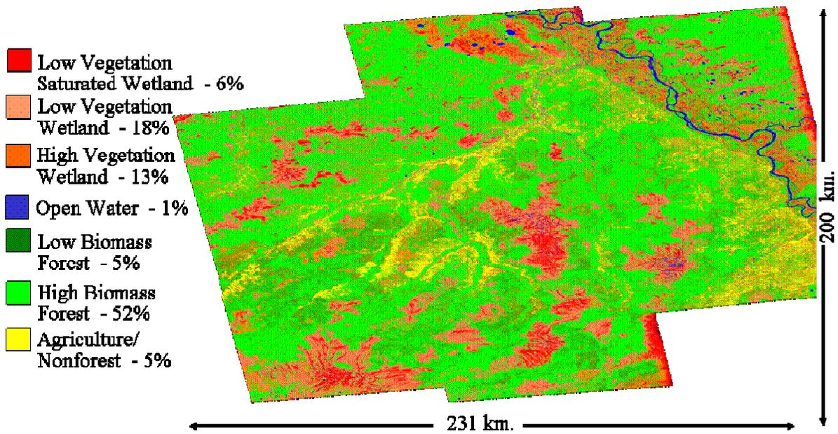
**Figure 11.** Landcover mapping for the Chaya Basin region, focusing on inundated wetland features and derived using ALOS PALSAR with Random Forest classification scheme applied. Landcover classes and the percent regional area covered by each are provided in the key.
