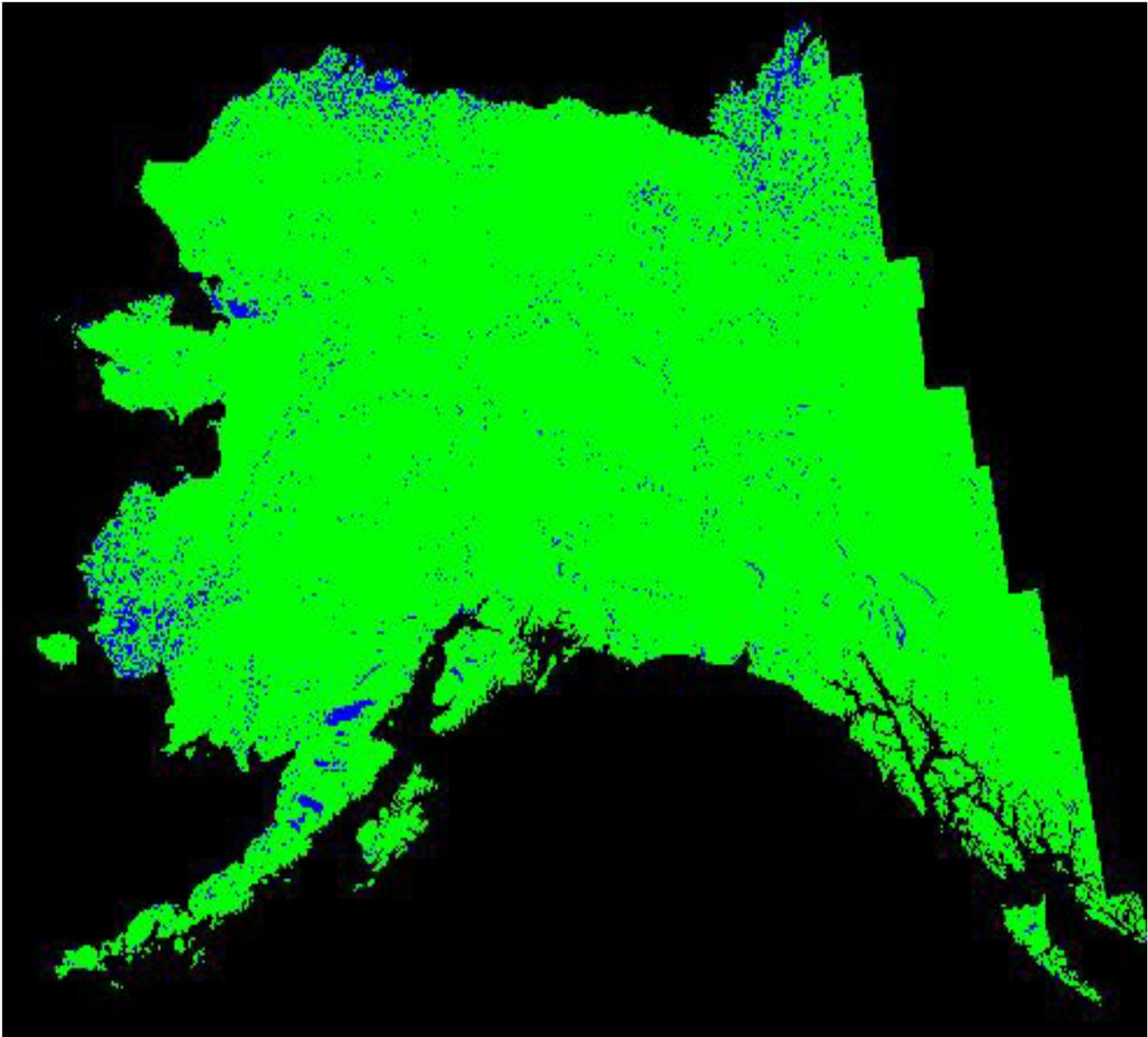
**Figure 2.** The open water map above was generated using an MLE supervised based approach applied to the Alaska JERS-1 summer mosaic. The product has spatial resolution of 100 meters. A DEM was used to mask out areas of high topography where radar shadowing was confused as open water.
