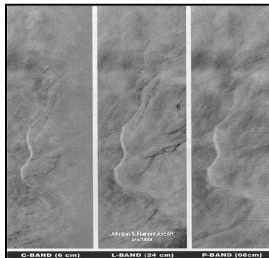
Fig. 2.3.8-2 Differences in sea surface representation according to SAR wavelength
