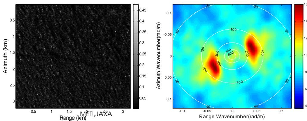
Fig. 2.3.8-5 High-resolution mode PALSAR sea surface image (left) and two-dimensional spectrum (right).
