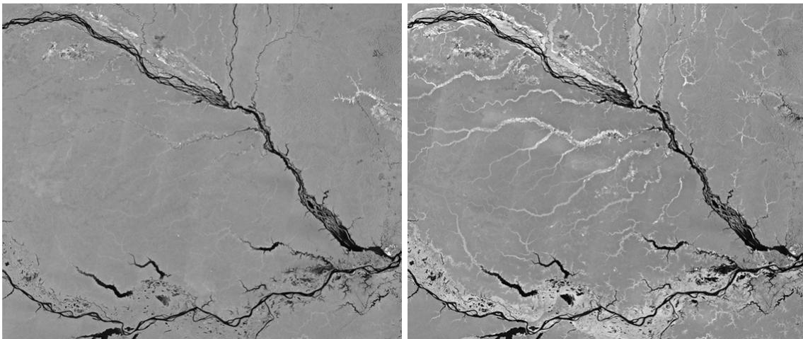
Figure 2.3.3-4 JERS-1 SAR (L-HH) sensitivity to forest inundation (left – Amazon basin at low water; right – high water). Bright areas - flooded forest, grey - non-flooded forest; black - open water.
