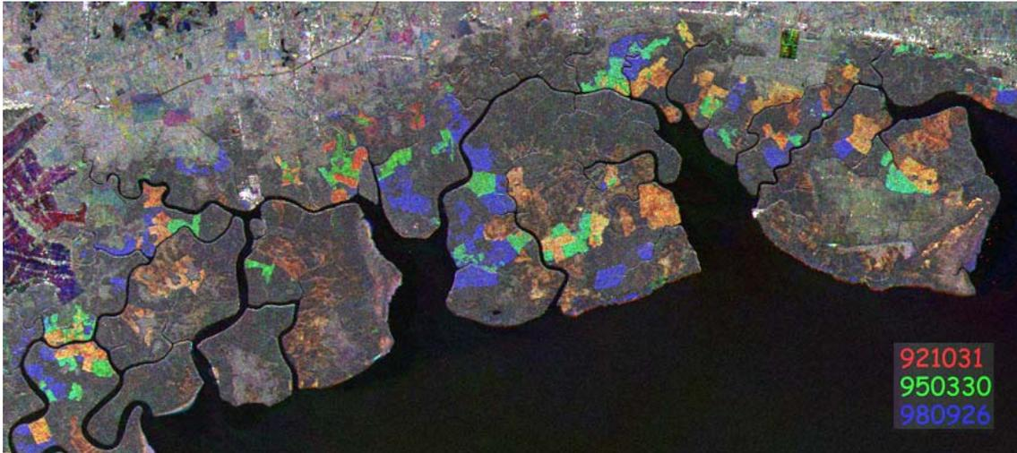
Figure 2.3.3-2 Disturbance monitoring of mangrove forest in Southeast Asia, using a multi-temporal time series of JERS-1 SAR data (Red:1992; Green:1995; Blue:1998). Undisturbed/mature mangrove appears in dark grey. Clearings which occurred 1992-1995 and 1995-1998 are green and blue respectively, while regenerating areas since 1992 appear orange.
