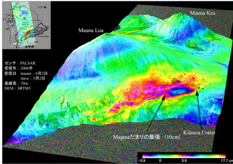
Fig. 2.3.4-2 Diastrophism detection at Kilauea Caldera, Hawaii Island, using PALSAR
