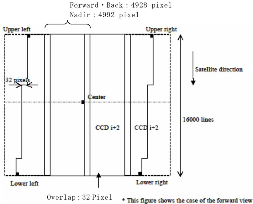
Figure 4.1.1-1 Concept of Scene Related Information for PRISM Uncorrected Image
