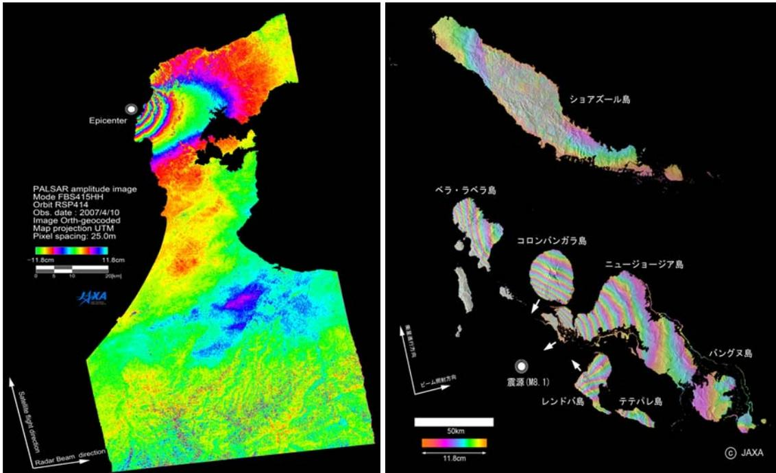
Fig. 2.3.6-1 Crustal deformation detected using differential interferometric technique of PALSAR data
