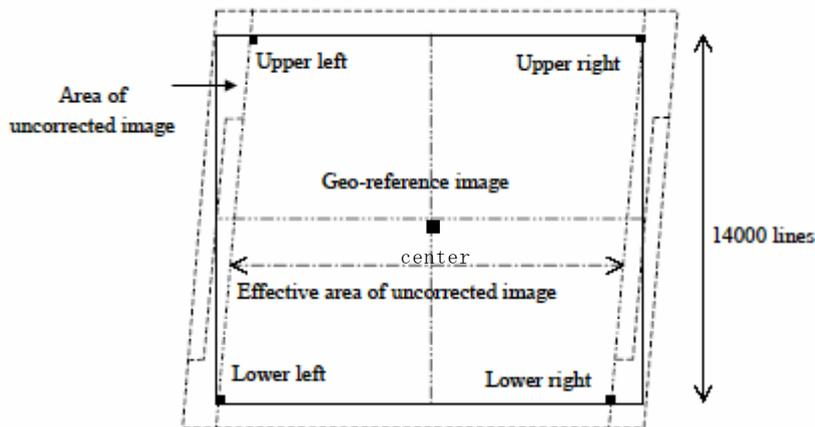
Figure 4.1.1-2-2 Concept of Scene Related Information for PRISM 1B2 Geo-reference Image
