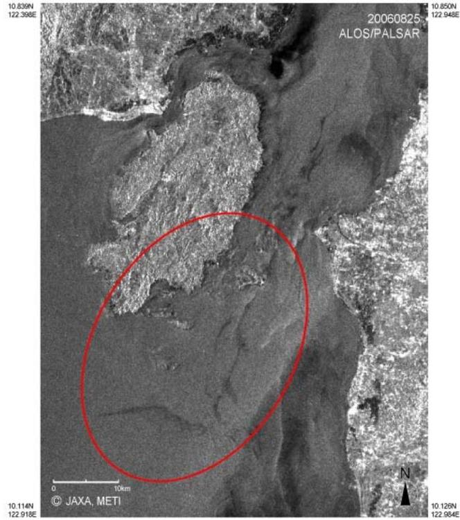
Fig. 2.3.6-3 PALSAR image of oil spill caused by tanker accident on August 11, 2006, near the island of Guimaras, Philippines (darker swath within red oval is believed to be leaked oil)
