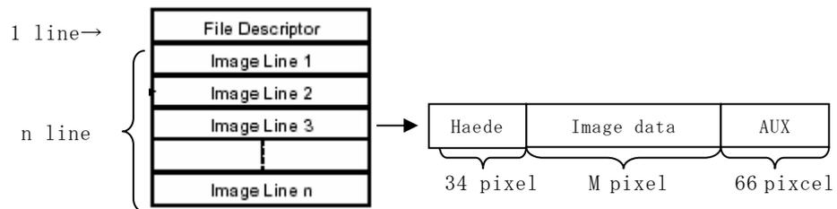
Fig. 4.2.2-1 The record structure of image file
