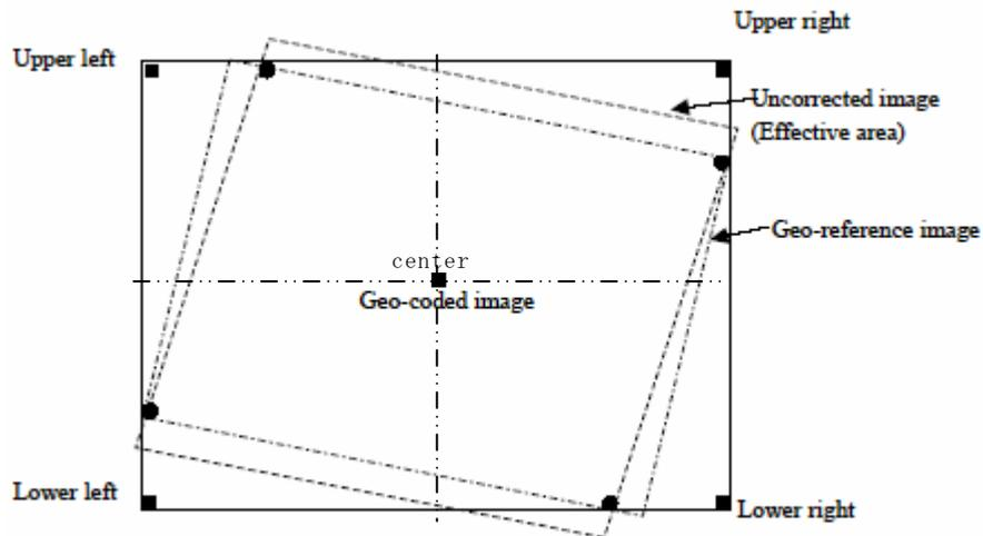
Figure 4.1.1-3 Concept of Scene Related Information for PRISM 1B2 Geo-coded Image
