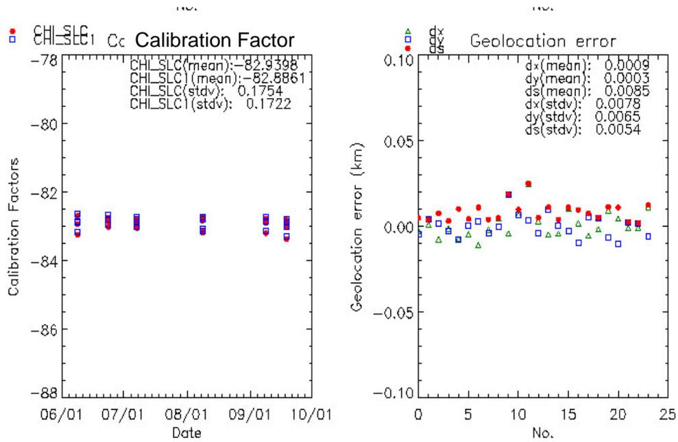
Fig. 2.3.1-1, Fig. 2.3.1-2 Time-based changes of radiometric accuracy Geometric accuracy distribution
