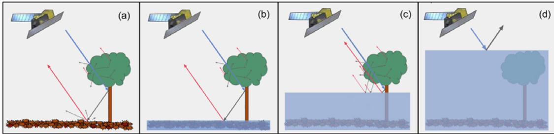
Figure 2.3.3-3. L-band (HH) backscattering mechanisms. Blue arrow – transmitted signal. Red - parts of the signal reflected back towards the satellite. Black – part of signal reflected away from the satellite.
