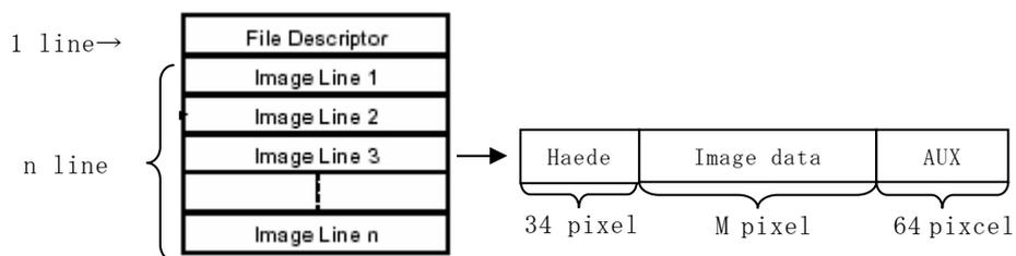
Fig. 4.1.2-1 The record structure of image file
